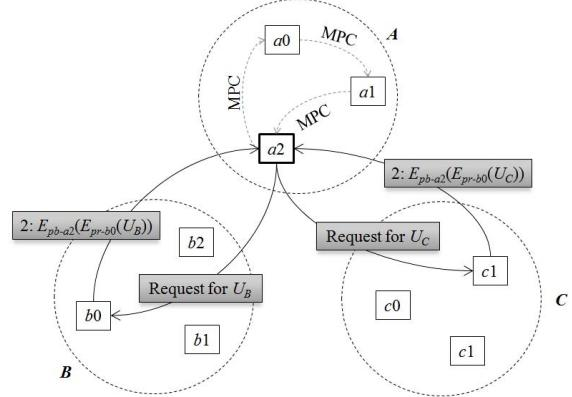
Fig. 5. The cluster based MPC technique
