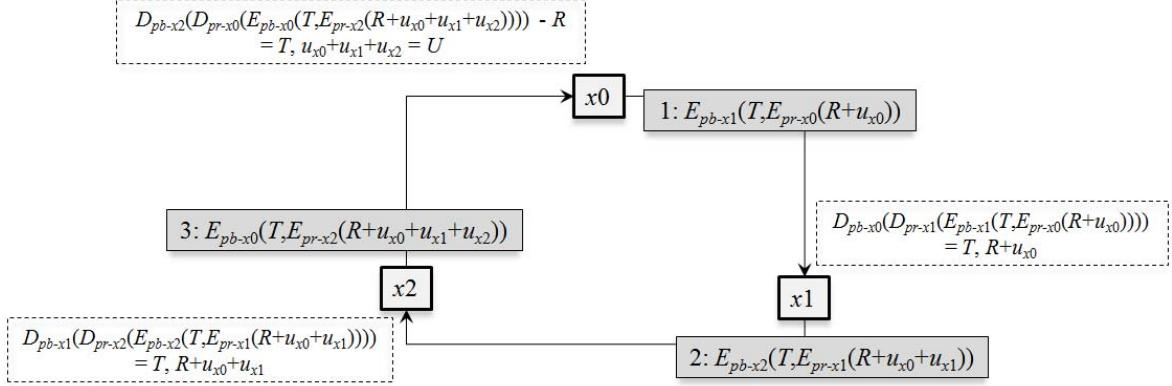
Fig. 4. The MPC technique for summing the usage vectors of the participating nodes that includes authentication and confidentiality security measures also.
