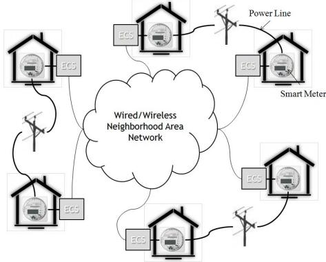
Fig. 1. The communication network between the smart meters.
